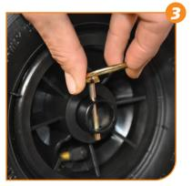
Fix the pin to block the wheel
