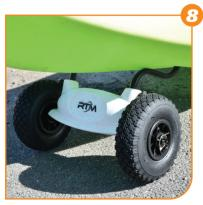
Place the cart under the kayak using the self-bailing holes.
